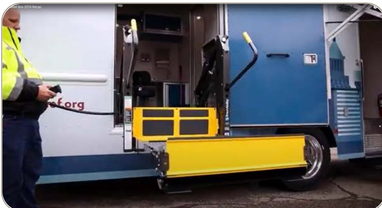
Handicapped accessible lift
